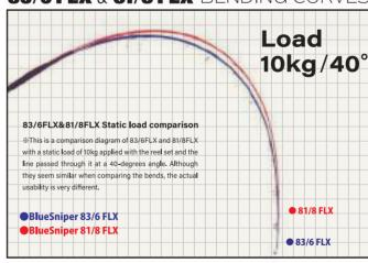
bends deeper as more load is applied to the blank, demonstrating high followability and tenacity. At the same time, the bending point moves closer to the hand, making it possible to reliably apply pressure to the fish while reducing physical strain.
