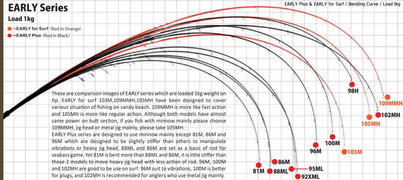
These are comparison images of EARLY series which are loaded 1kg weight on tip. EARLY for surf 103M,109MMH,105MH have been designed to cover various situation of fishing on sandy beach. 109MMH is more like fast action and 105MH is more like regular action. Although both models have almost same power on butt section, if you fish with minnow mainly please choose 109MMH, jig head or metal jig mainly, please take 105MH.
