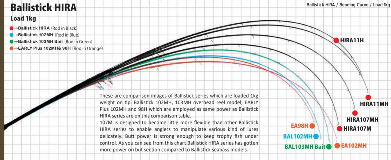
These are comparison images of Ballistick series which are loaded 1kg weight on tip. Ballistick 102MH, 103MH overhead reel model, EARLY Plus 102MH and 98H which are employed as same power as Ballistick HIRA series are on this comparison table.
