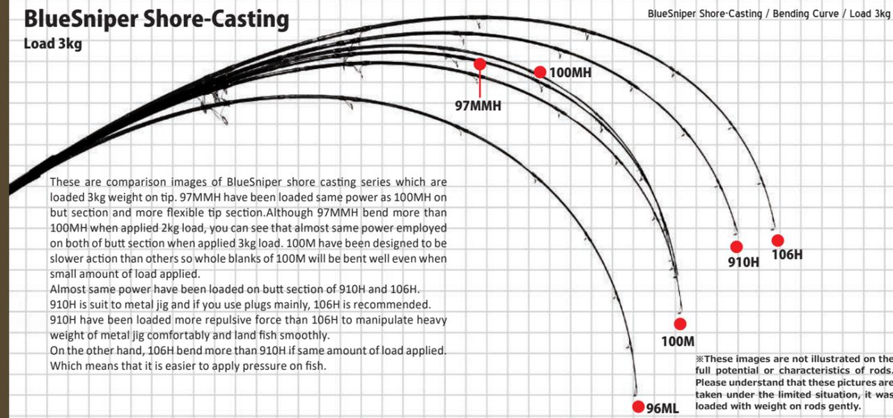
These are comparison images of BlueSniper shore casting series which are loaded 3kg weight on tip. 97MMH have been loaded same power as 100MH on butt section and more flexible tip section. Although 97MMH bend more than 100MH when applied 2kg load, you can see that almost same power employed on both of butt section when applied 3kg load. 100M have been designed to be slower action than others so whole blanks of 100M will be bent well even when small amount of load applied.
