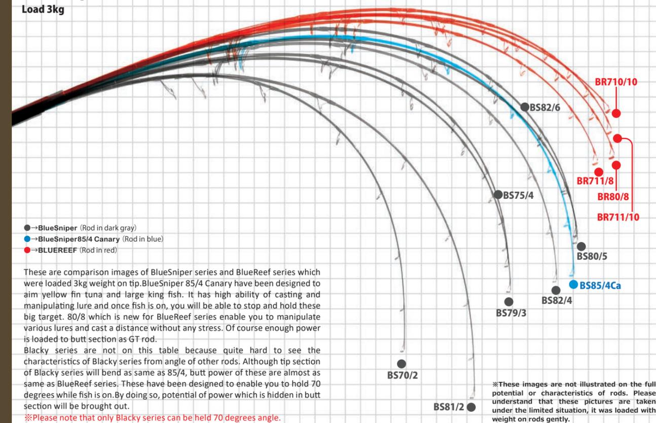
These are comparison images of BlueSniper series and BlueReef series which were loaded 3kg weight on tip. BlueSniper 85/4 Canary have been designed to aim yellow fin tuna and large king fish. It has high ability of casting and manipulating lure and once fish is on, you will be able to stop and hold these big target. 80/8 which is new for BlueReef series enable you to manipulate various lures and cast a distance without any stress. Of course enough power is loaded to butt section as GT rod.
