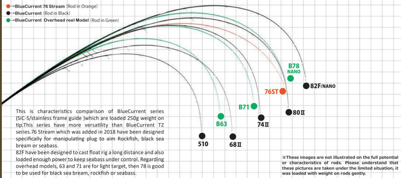
This is characteristics comparison of BlueCurrent series (SiC-S/stainless frame guide) which are loaded 250g weight on tip. This series have more versatility than BlueCurrent TZ series. 76 Stream which was added in 2018 have been designed specifically for manipulating plug to aim Rockfish, black sea bream or seabass.
