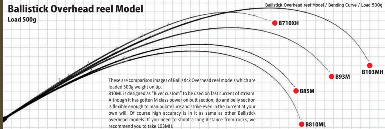
These are comparison images of Ballistick Overhead reel models which are loaded 500g weight on tip. 810ML is designed as "River custom" to be used on fast current of stream. Although it has gotten M class power on butt section, tip and belly section is flexible enough to manipulate lure and strike even in the current at your own will. Of course high accuracy is in it as same as other Ballistick overhead models. If you need to shoot a long distance from rocks, we recommend you to take 103MH.
