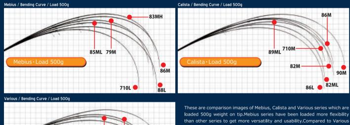
loaded 500g weight on tip. Mebius series have been loaded more flexibility than other series to get more versatility and usability. Compared to Various series, Mebius series have been designed to become softer.
